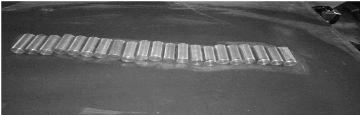
Fig. 2. Sample of the mild steel (EN10) test pieces.
